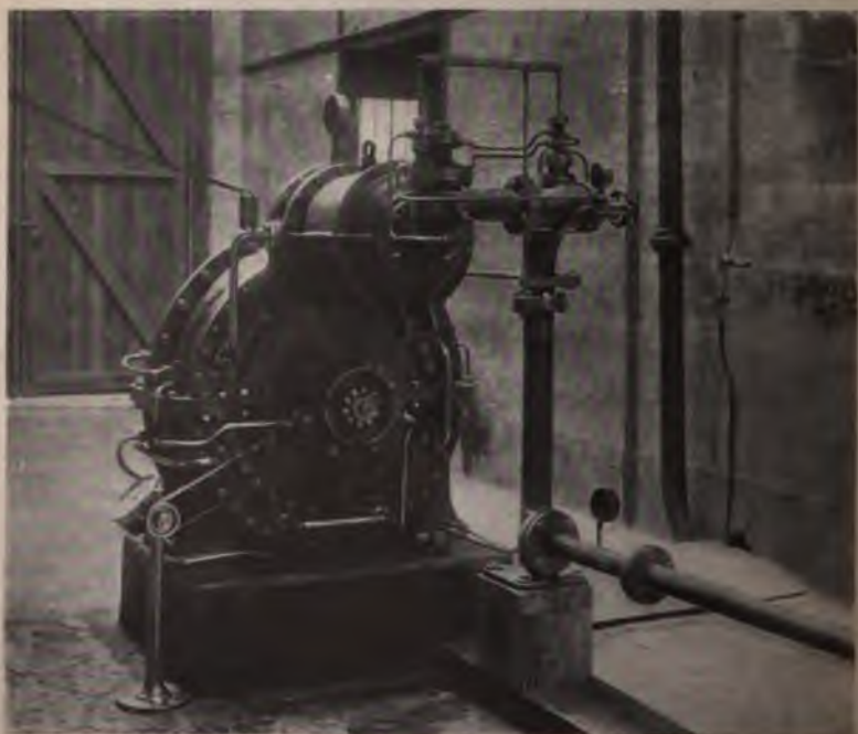
FIG. 85.—The Armengaud and Lemale gas turbine. Another view of the combustion chamber, with air and fuel connections.
